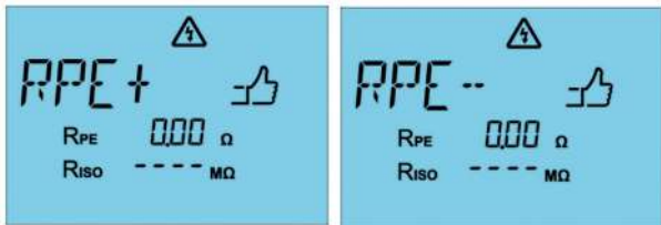
Fig. 56: R_{PE+} → positive current direction (left) and R_{PE-} → negative current direction (right)
