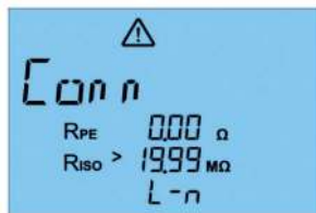
Fig. 45: Check the connection of the current-carrying conductors
