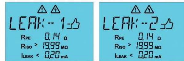
Fig. 23: Measurement of the protective conductor current on both sides
